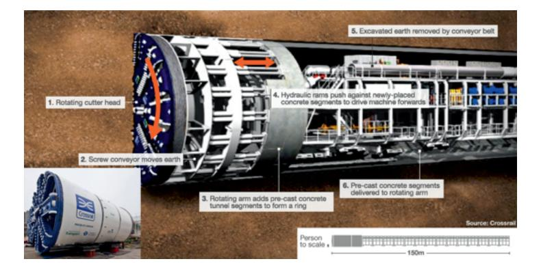
Tunnel Boring Machines are used to excavate through earth to make tunnels for the transport of people, energy, information, water, etc.
